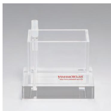
Dedicated tank for Erichsen test. Also convenient for other experiments and trial plating to fine parts. An air agitation pipe include this product.
