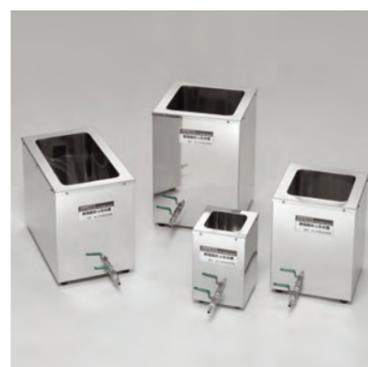
Standard stainless-steel (SUS316) and double-walled plating tank used for electroless nickel plating. Since double-walled structure, its excellent heat retention property enables to conduct high-temperature experiment up to 95°C. For electroless plating of materials other than nickel, tanks made of other materials are recommended. Please contact us for further details. Compatible heaters: 300W stainless steel heater (A-50-KH03300), 500W stainless steel heater (B-84), 500W quartz heater (B-95-1A)
