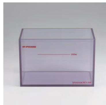
A tank which enables to perform simple experiments more easily and accurately with relatively small liquid volume. Fixing anode and cathode is easier and user-friendly. Variety of optional parts are also available such as anode plates with exact size, cathode rocker, and so forth. Please refer to p77 for the combination example. We also manufacture a tank with heater slit on the bottom for special order. Compatible Heater: Wafer Tank Heater (A-52-ST4-P10A/P10WA/P10WJA)
