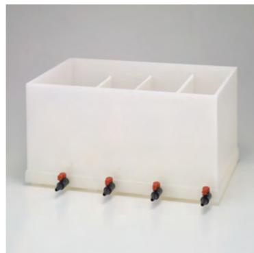
PP rinse tank divided into four partitions. By supplying the first and second tank water to the plating bath during use, waste-water can be effectively reduced. Only the water in the final tank is circulated for use through ion-exchange.
