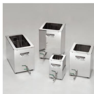
Stainless-steel (SUS316), double-walled plating tank used for electroless nickel composit plating. Since doublewalled structure, its excellent heat retention property enables to conduct high-temperature experiment up to 95°C. Tank with a boat-shaped structure inside to improve stirring efficiency (see figure on the right). The corresponding size is 2 to 20L.
