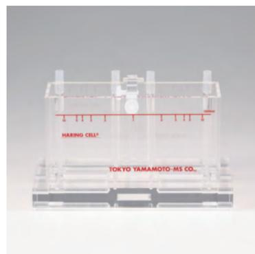
Dedicated tank for measuring macro throwing power. Also convenient for other experiments and trial plating to micro parts. Various busbars, anode plates, and jigs, recommended to make experiments easier to perform, are available.
